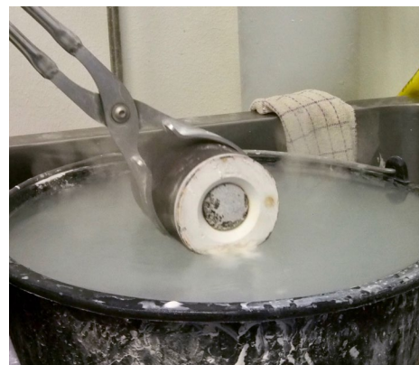
Quench and devest the flask by submerging it in water.
