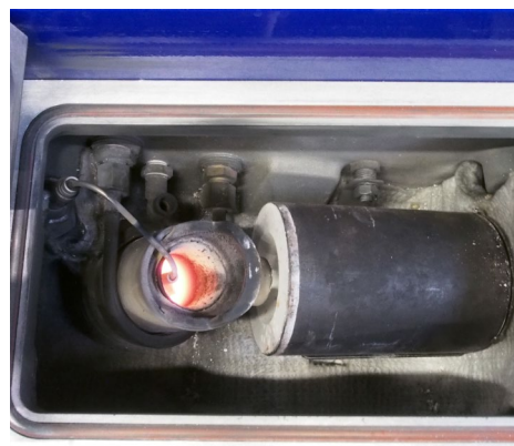
Vacuum or centrifugal casting methods improve fill to thin details.
